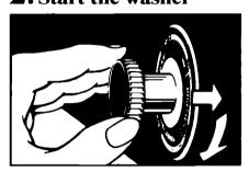
A. Push in the Control Knob and turn it to the right (as indicated by the arrows shown above). It must be pushed in and turned only clockwise.
